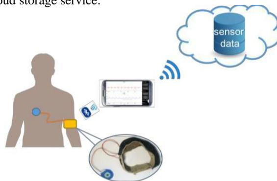
**Figure 3. Illustration of a cloud-enabled wearable system for monitoring multiple physiological signals continuously.**
