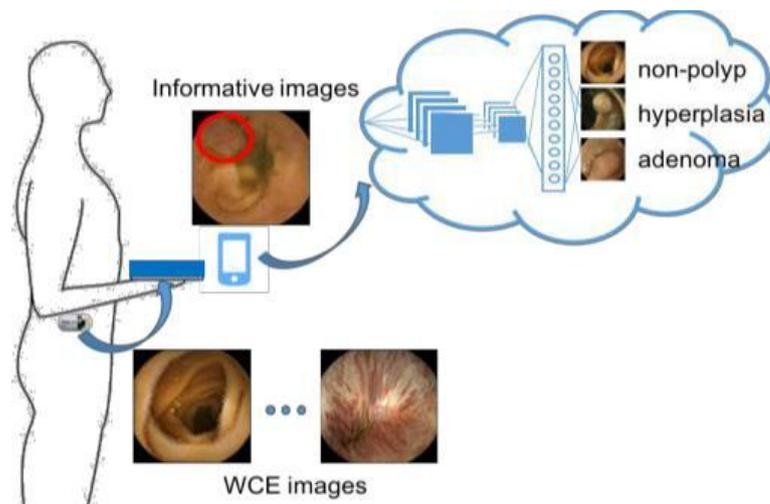
**Figure 2. Illustration of a cloud-enabled WCE system for screening and classification of colorectal polyps.**
